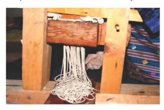
pushed down, the paste in the central box is squeeze out through the multiple holes in the bottom in the shape of noodles.
